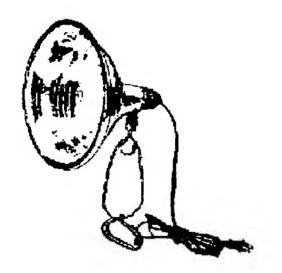
4. If your lamp has a painted interior, the Light output can be increased considerably by gluing aluminum foil to the inside of the reflector bowl. Keep the foil an inch or so from the bulb end of the reflector. Do not be concerned if the foil is not smooth when finished. The following illustrations are for an 8" reflector lamp, and 8x10" filters. For
